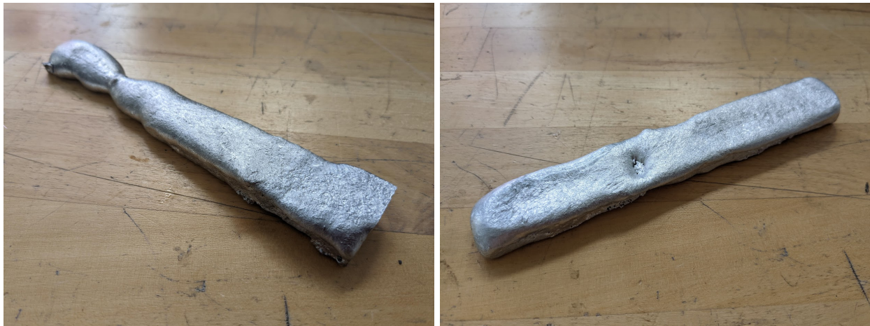
Casting Results 356 on left, 6000-series on right
